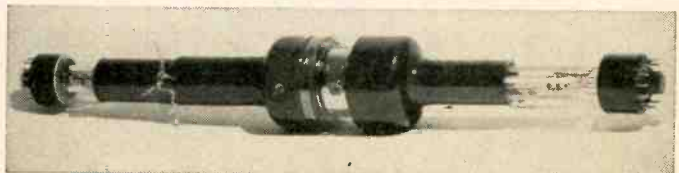
Scan-conversion tube that changes PPI display into TV image.
